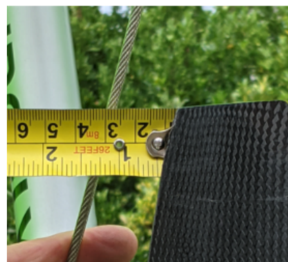
Manually deflected wire
