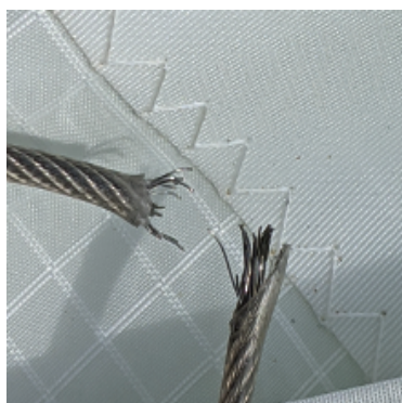
Sheared rear wire
