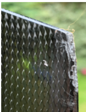
Damaged propeller tip
