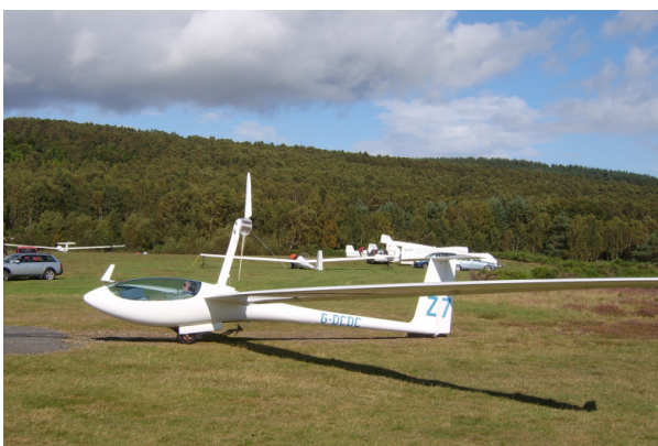
John Williams about to launch in his electric-powered self-launched Antares (photo: Diana King)
